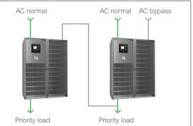
Live standby redundancy
