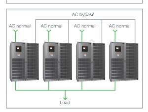
Distributed parallel connection for increased power and redundancy
